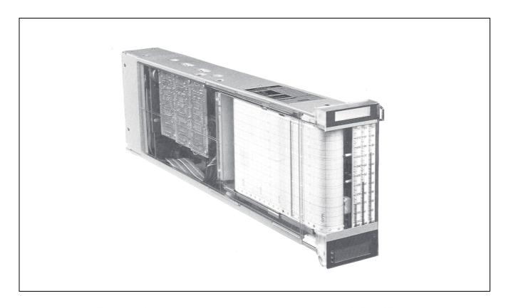
This instrument receives one, two, or three 4 to 20 mA, 1 to 5 V, or 0 to 10 V dc analog input signals, continuously records them on a 100 mm (4 in) rectilinear chart, and also displays them on 100 mm (4 in) vertical ribbon indicator scales. This recorder is often mounted side-by-side with 760 and 761 Series SINGLE STATION MICRO™ Controllers when recording is a requirement for their signals.
