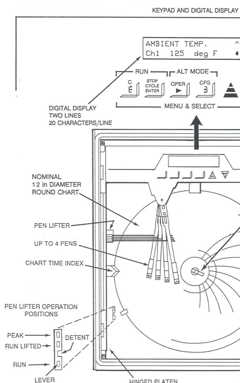
Figure 1. Figure 1. Recorder with Front Door Removed
